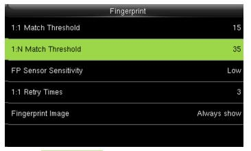
Here select 1:N match threshold value is the similarity of verification and the enrolled template.
