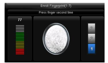
Place the same finger on the fingerprint sensor for the second time.
