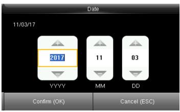
You can set the date by using the keypad. Here the date is set to 11/03/2017.
