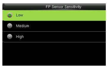
The default value Medium is recommended. You can set the sensitivity of fingerprint collection to High when the response to finger scan lags in a dry environment. When the usage environment is humid, you can set the sensitivity of fingerprint collection to Low if the fingerprint is difficult to identify.
