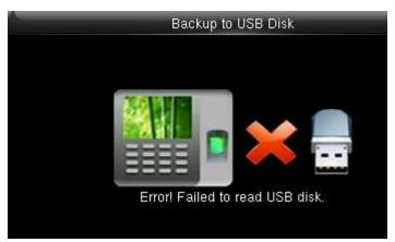
If the usb is not properly inserted the above scdreen will be displayed. You can either change the USB or insert it properly again.
