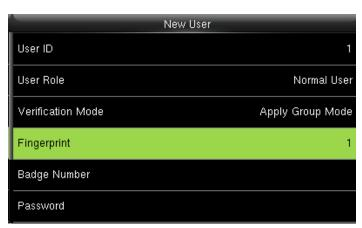
After the fingerprint is enrolled successfully the fingerprint will be shown as 1 as above which means one fingerprint is enrolled.
