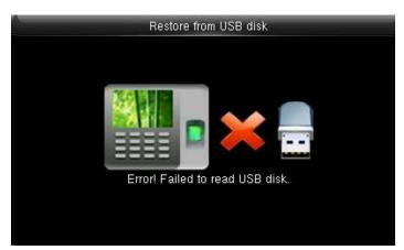
If the USB disk is not properly inserted the above scdreen will be displayed. You can either change the USB or insert it properly again.
