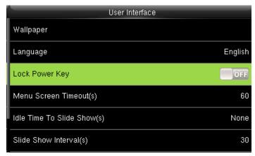
To prevent hostile power-off, select whether to lock power-off or not. "disable": the power is off 3 seconds after pressing power-off.
